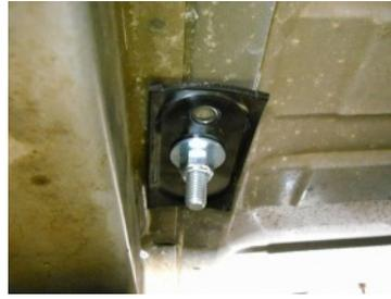
This photo is the under-floor view of the seat belt bolt and nut. Use the supplied backing plates under the floor as shown.
