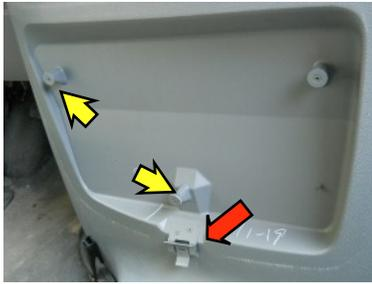
Remove the console from the motorbox cover by reaching under and pressing down on the clip (red arrow) and lifting up on the console. Then remove the clip by drilling out the rivets with a 1/8" drill. Also remove the 2 screws (yellow arrows). Discard the screws and the clip.
