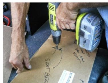
Once the holes are marked, pre drill with a 3/16" drill bit and finally with a 1/2" drill. There's a wire under the mat near the drilling locations which should not be a factor, but check under the mat and under the van floor before drilling anyway. Be sure to vacuum up all the metal chips you produced while drilling.
