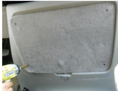
Included in the kit is an upholstered panel that fits in the recessed area where the console was located. There are holes on the back side of the upholstered panel that land over the protrusions on the fiberglass motor cover. Align the upholstered panel over the protrusions and mount the panel onto the motor box with the 2 shorter screws on the driver side and the 2 longer screws on the passenger side (snug, but do not overtighten) the screws.
