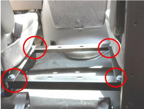
Install the cross rails onto the side rails as shown in the photo at left. Make sure that the cross-rails are mounted UNDER the side rails (red circles).
