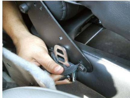
Once the seat assembly is bolted to the brackets, feed the seat belts up through the elastic straps attached to the side of the seat hinges
