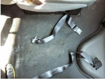
The seat belts are installed such that the buckle end is next to the driver seat and the adjustable end is next to the passenger seat.
