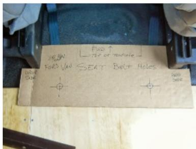
Also inside the mounting kit, you will find the cardboard template for the seat belts. Set the floor template down as shown in the photo at left. Mark the floor with a white grease pencil or other suitable marker at the locations on the template for the seat belt bolts. Please **check for obstructions** under the van floor and under the mat before you center-punch and drill the 1/2" holes needed. (Please disregard the plywood flooring shown in the photo).
