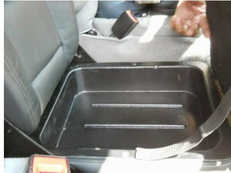
Flip up the lower seat cushion to reveal the plastic tray. Remove the tray and screw holding the nylon strap.
