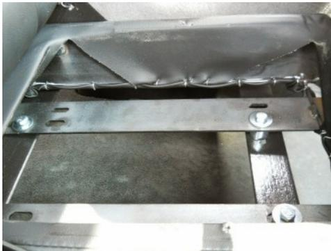
With the tray removed, the bolts and spacers used to attach the seat assembly to the brackets are visible. Use the supplied spacers to adjust the height and angle of the 3<sup>rd</sup> man seat to your satisfaction.
